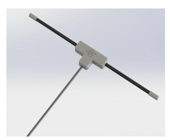
Mount the antenna with the elements as far as possible from carbon fiber, or other materials, and somewhere with a good view of the ground-based Tx for most model orientations.
